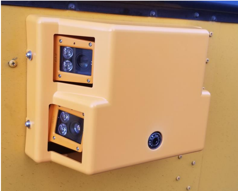
A close up view of camera system with license plate reader and OverWatch video camera.
